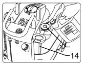
Indicator is light: insufficient "No Scale" Indicator is dark: sufficient "No Scale"
